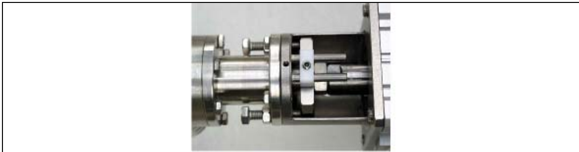
Figure 3.4. KS/6 stroke limited by bolts. Piston is out in this position.
