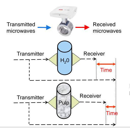
Microwaves travel faster in pulp than in water.
