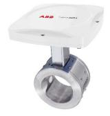
Consistency measurement is based on the detection of speed variations in pulp slurry. Speed variation is detected with true-phase measurement.
